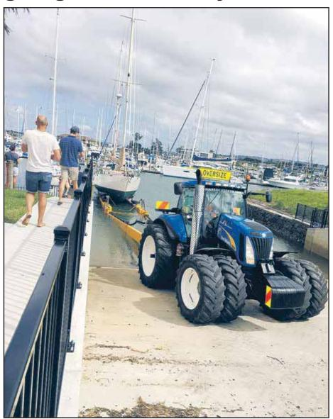
Rod and Jo Scott's yacht Long White Cloud being backed into the water by the Mardsen Marina's custom built hydraulic slipway trailer after undergoing maintenance at the new Marsden Cove haul out facility.
