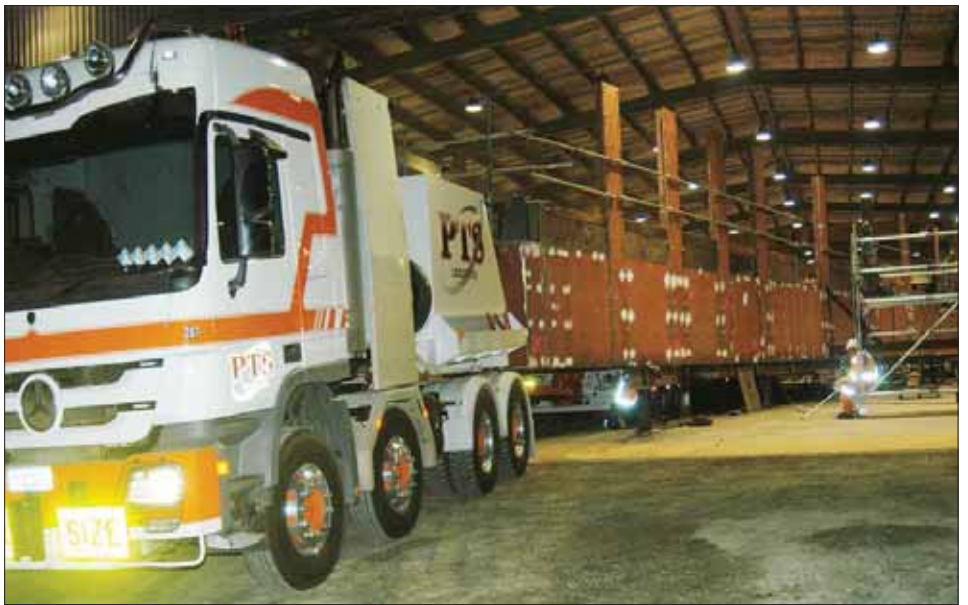
The 40 - metre - long pontoon is loaded onto a truck at the SPIIND workshop for transportation to the port
